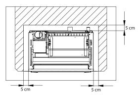
For correct functioning of the insert, during construction of the flue the measurements between the insert and internal walls of the flue must be respected (figure below).
