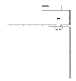
The 2 side frames are fixed to the upper frame by means of 2 screws each side.
