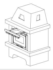
The optional pellet feeding kit allows pellets to be fed into the feedbox from the front without having to extract the insert (operation that requires machine switch-off).
