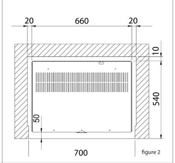
For the insert to operate correctly, a **minimum** side and rear space must be guaranteed, as shown in figure 2; the coatings must be made of **non-flammable** material.
