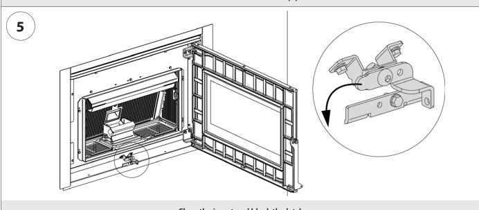
Close the insert and block the latch.
