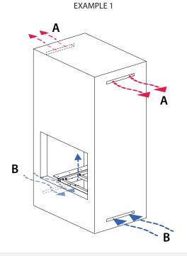
**A**: Air convection outlet. Minimum section 120cm<sup>2</sup>. **B**: air inlet from room. Minimum section 120cm<sup>2</sup>.
