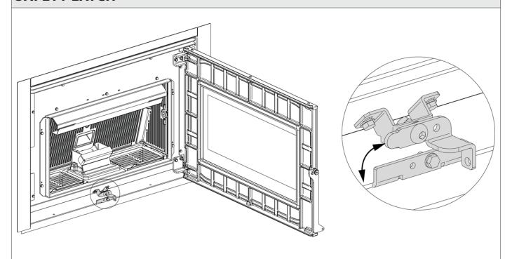
Use the poker supplied to perform the release/block operation. (Turn clockwise to release and anti-clockwise to block).
