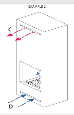
**C**: Air convection outlet. Minimum section 240cm<sup>2</sup>. **D**: air inlet from room. Minimum section 240cm<sup>2</sup>.
