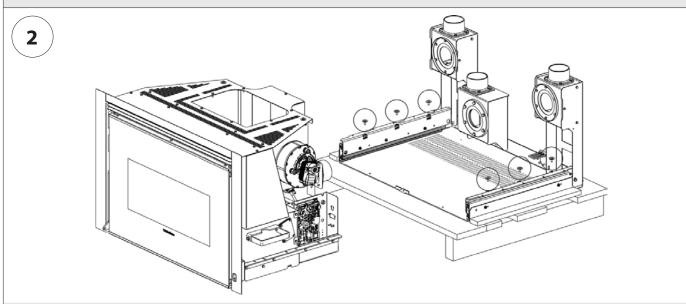
Remove the 6 screws and remove the flue pipe from the base.
