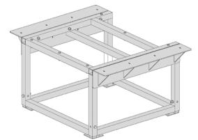
If there is no pre-existing chimney, one can be built using an insert-holder pedestal (optional kit). In fact, the latter fixes the insert to the ground.
