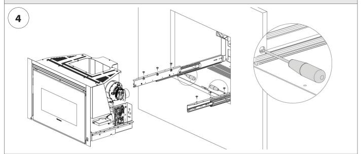
Block the rails with two screwdrivers and secure the flue pipe to the base with 6 screws.
