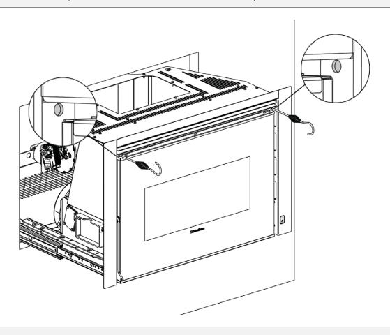
Holes present on two sides for the extraction of the insert via pokers.
