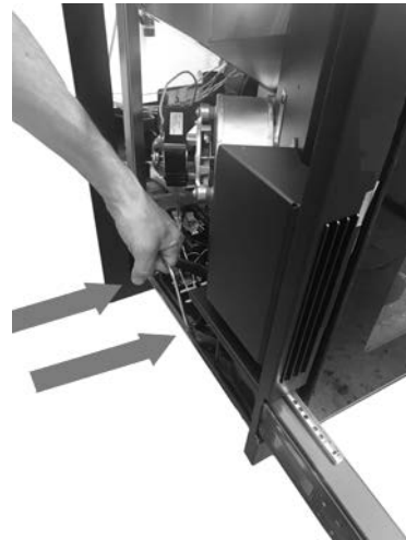
Fig. 23 - Machine body removal
