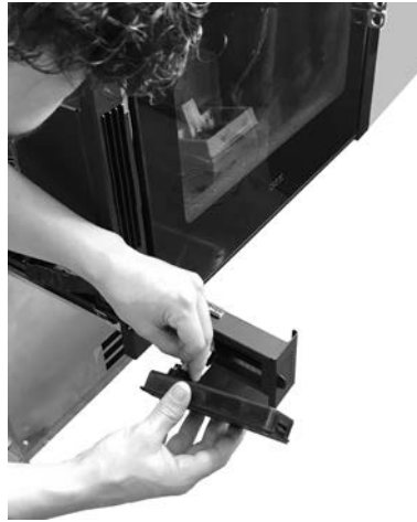
Fig. 79 - Remove the flat cable
