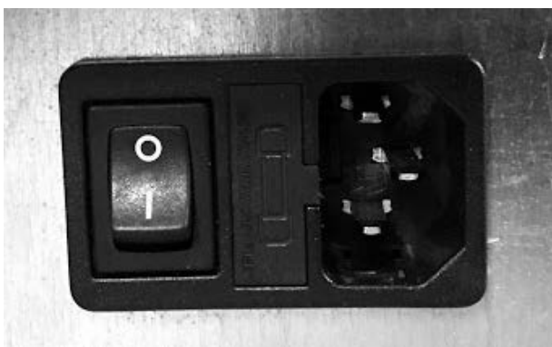
Fig. 27 - Electric socket with master switch
