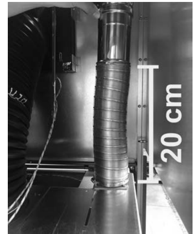
Fig. 48 - Flexible pipe connection (rear view of the insert)
