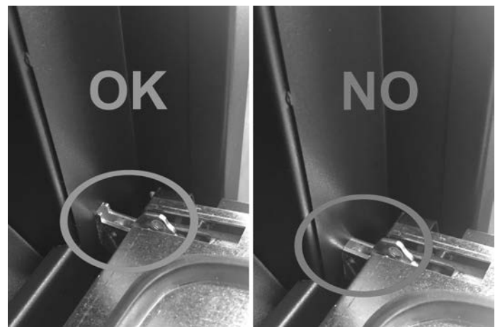
Fig. 69 - Correct hooking of the hinge
