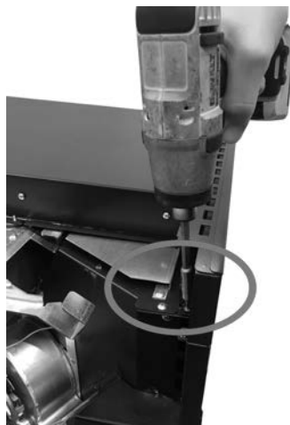
Fig. 54 - Drawer front fixing
