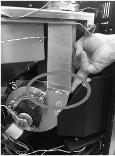
Fig. 46 - Seal with adhesive aluminium tape
