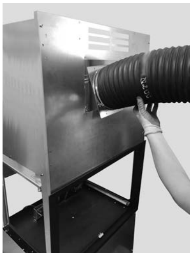
Fig. 64 - Flexible hose positioning
