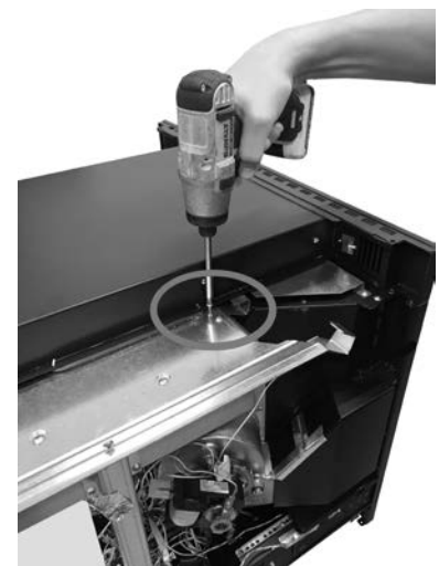
Fig. 55 - Drawer central fixing
