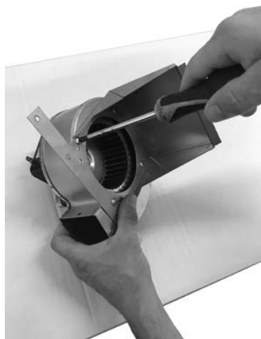
Fig. 41 - Remove the screws
