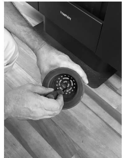
Fig. 37 - Burning pot cleaning
