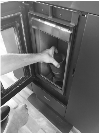
Fig. 35 - Burning pot extraction
