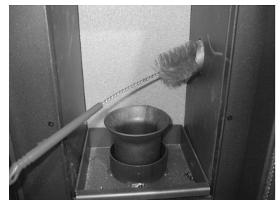
Fig. 40 - Cleaning with a brush
