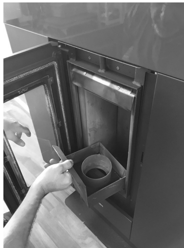
Fig. 36 - Burning pot cleaning
