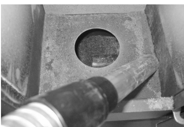
Fig. 38 - Ash tray box cleaning
