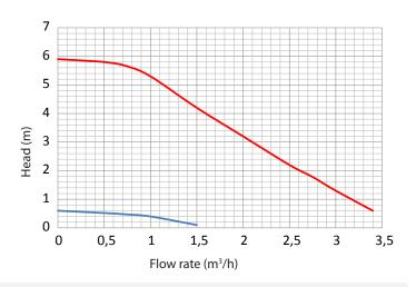
The diagram at the side illustrates the behaviour of the pump used on our thermo-products at the speeds that can be set.
